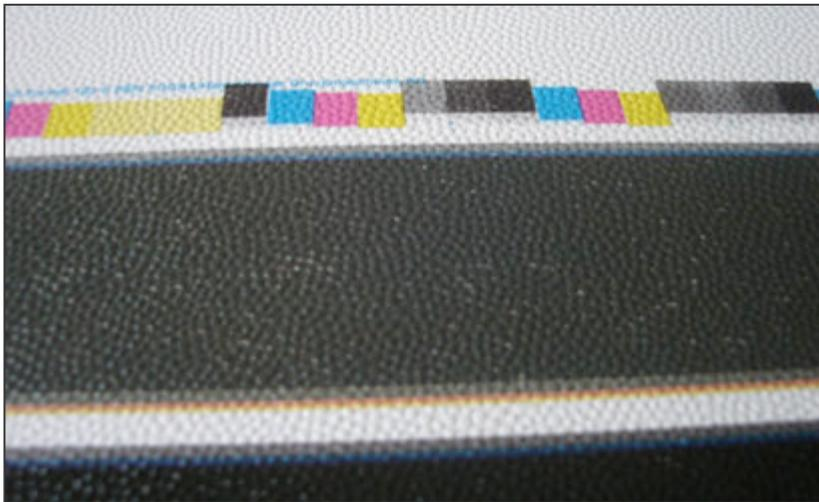
Excessive printing pressure (impression) register is lost
